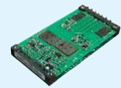
VWS150 Industry Standard Full-Brick 4.60 x 2.40 x 0.50 inch 116.8 x 61.0 x 12.7 mm
