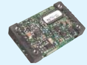
QBS Industry Standard 1/4-Brick 2.30 x 1.45 x 0.5 inch 58.42 x 36.8 x 12.7 mm
