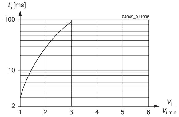
Fig. 6b Typical hold-up time t_h versus relative AC input voltage (LS models)
